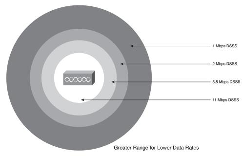
The following outlines the characteristics of data rates as they apply to client devices and signal strength:
