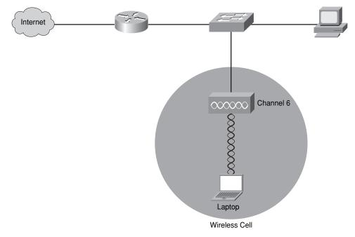
If a single cell does not provide enough coverage, any number of cells can be added to extend the range. This range is known as an Extended Service Area (ESA). Figure 3-10 shows an ESA topology.
